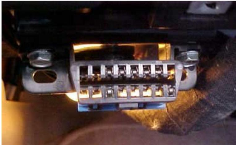
Figure 2 – The datalink connector (DLC) for OBD-II vehicles
