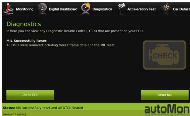
Figure 11 – View after resetting the MIL and clearing DTCs
